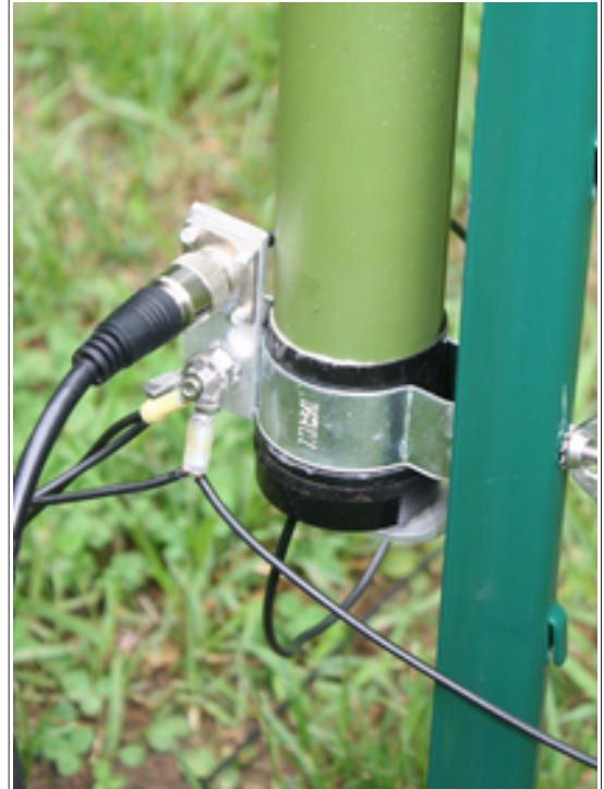
Here is a closer look at the radial attachment and coaxial feed attachment.
