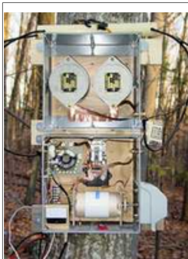
Getting on 2200 meters can be a bit more involved than getting on 630 meters. This LF antenna tuning unit was constructed by John Andrews, W1TAG/WD2XES.
