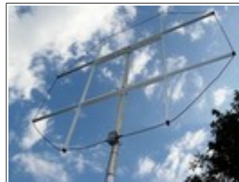
WD2XSH Experiment participant Ralph Wallio, W0RPK, employs a homebrew shielded loop for receiving on 630 meters.
