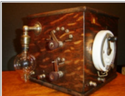
The de Forest Audion in its natural habitat, installed in a de Forest Audion Receiver. [Bob Allison, WB1GCM, photo]
